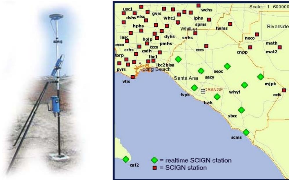
**A progressive RTK network in California deems the setting up of a base station a thing of the past.**
